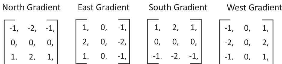
Fig. 2. Gradient filters used in our study.
